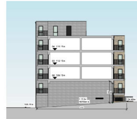
06. Section through Vehicular Access Ramp 1 : 200
